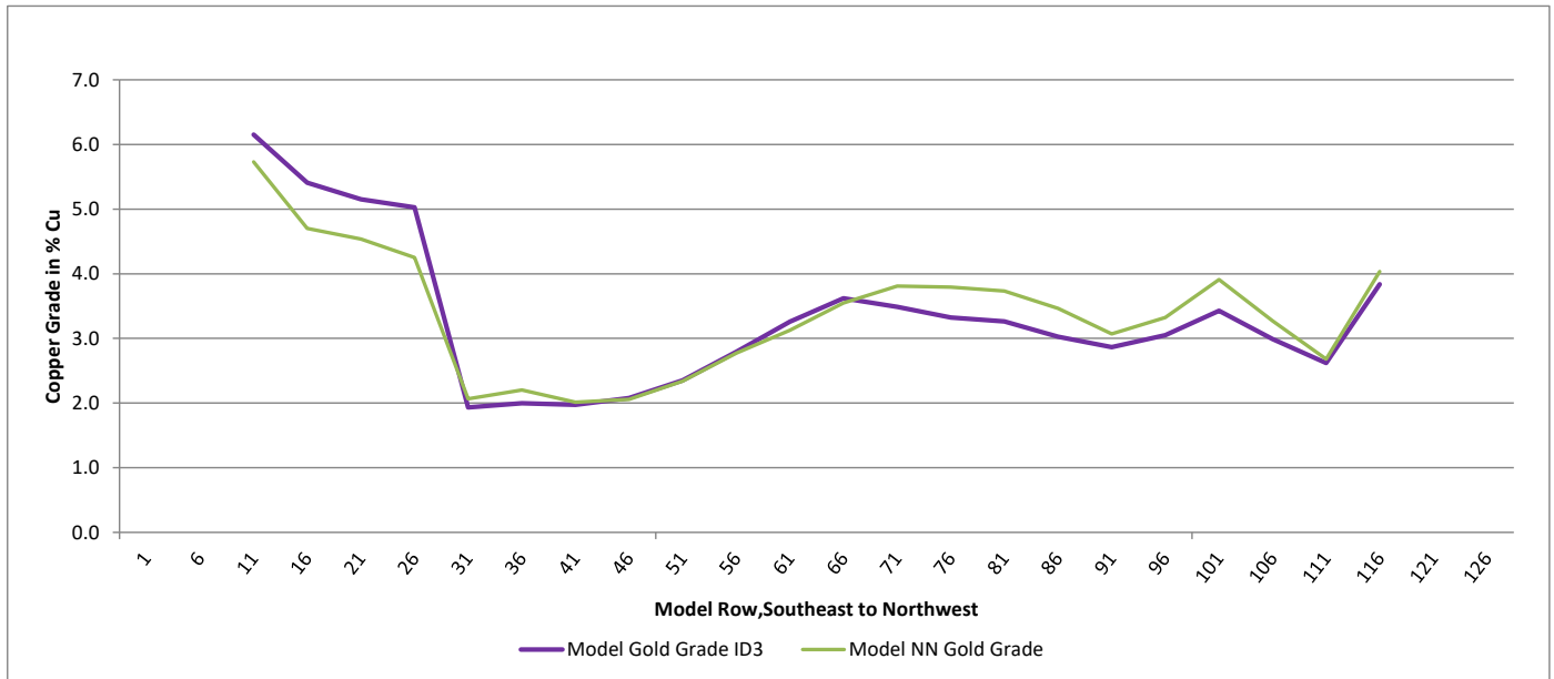
Figure 14-27: Cross Section Swath Plot for Gold, Inside the Grade Boundary
