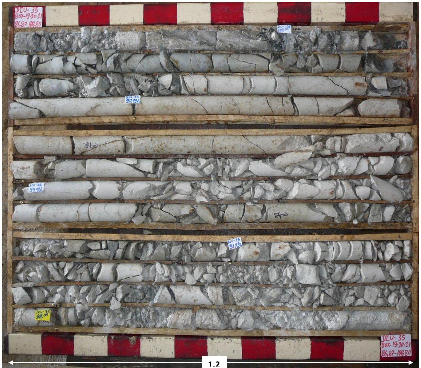
Figure 16-4: Rock Quality Adjacent to Piedras Blancas Regional Fault
