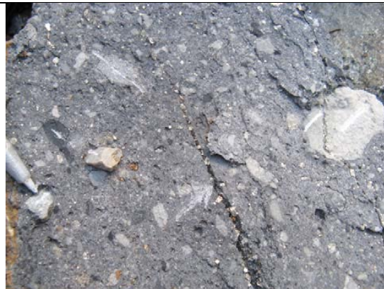
Photo 7. Texture of breccia with volcanic, sedimentary, and altered fragments, and a muddy dark matrix (Brechas Negras), derived from comminution of black shale
